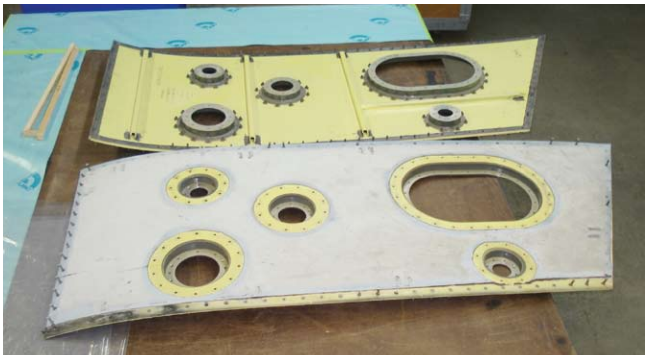
The existing SWUAP panels have a slight fore-and-aft curvature, and are composed of 50 plies of unidirectional carbon fiber.
